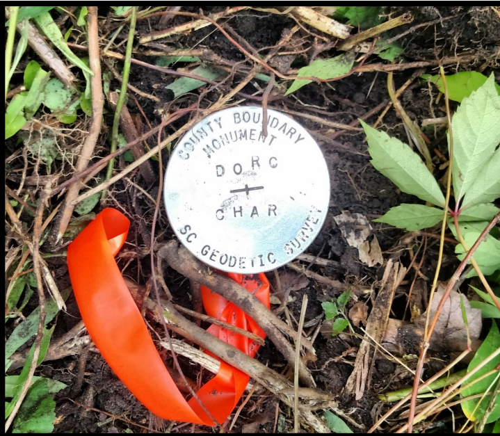
Corner Set is an approximately 3 foot long, 1 inch diameter rebar topped with a 4 inch stamped cap.
