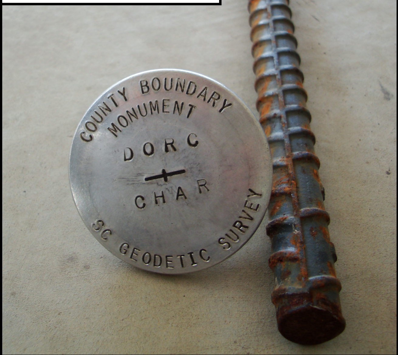
Corner Set is an approximately 3 foot long, 1 inch diameter rebar topped with a 4 inch stamped cap.
