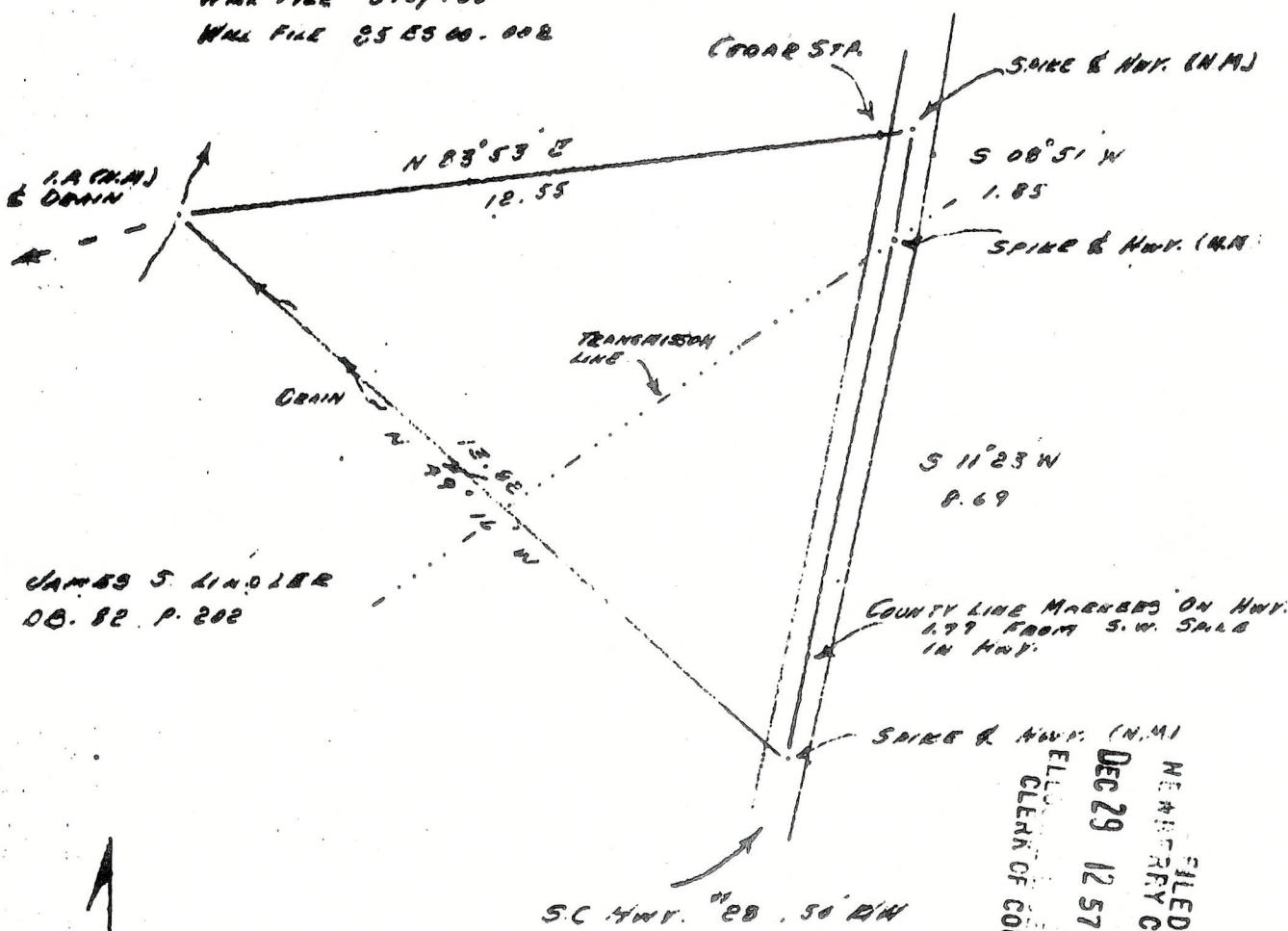
I hereby certify that the ratio of precision of the field survey is 1:600 as shown hereon and the area was determined by DMD Method of area calculation.
