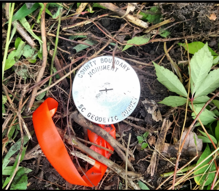
Corner Set is an approximately 3 foot long, 1 inch diameter rebar topped with a 3-½ inch stamped cap.
