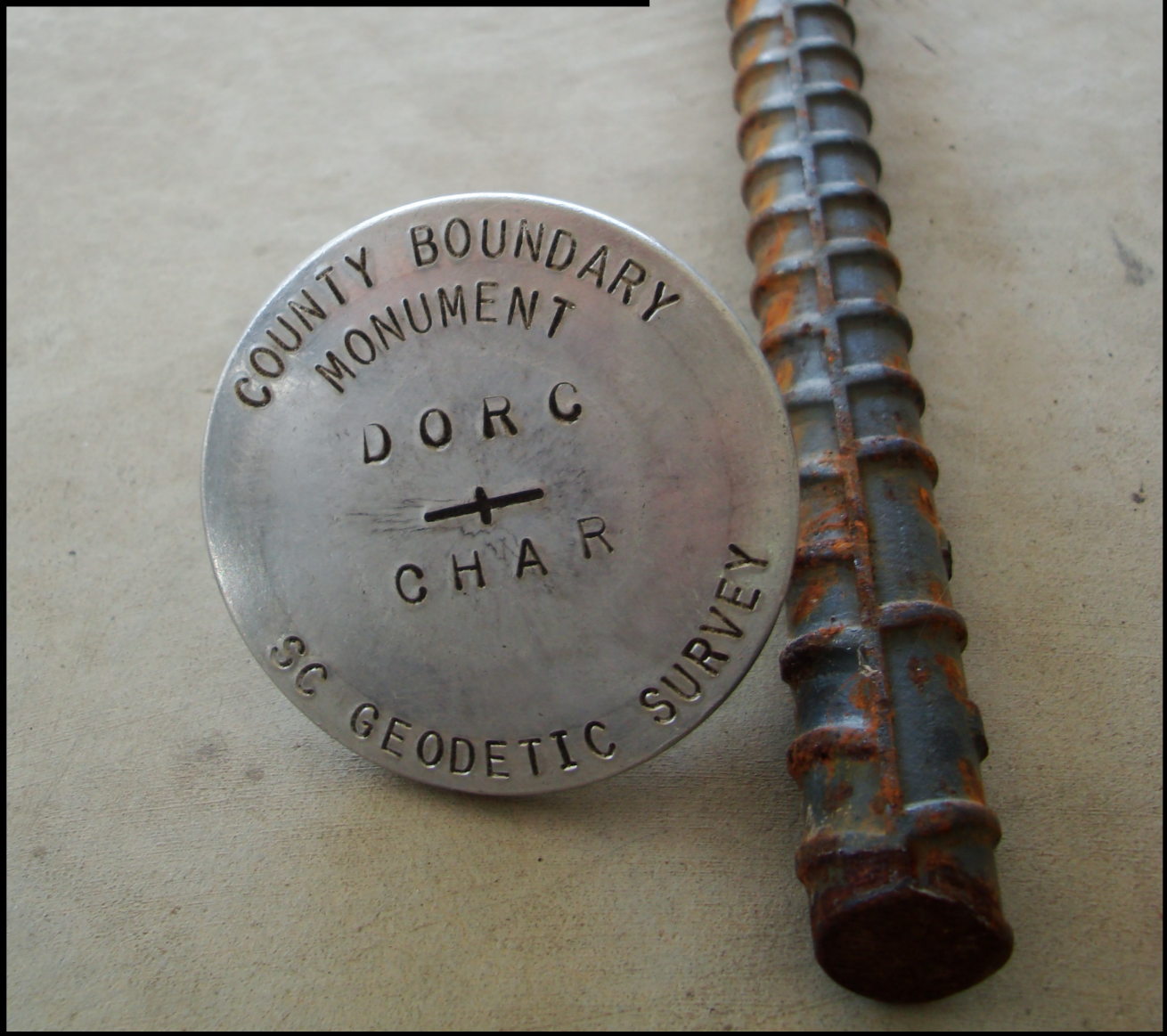
Corner Set is an approximately 3 foot long, 1 inch diameter rebar topped with a 3-½ inch stamped cap.
